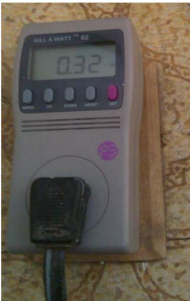
It is best to capture the cycling of these active and passive stages over a representative period of time as is done with refrigerators and water heaters. A less accurate means of calculating wattage when “on” would be to record the most common wattage (active or passive) or take the average of the active and passive wattages if they are not too far apart.
